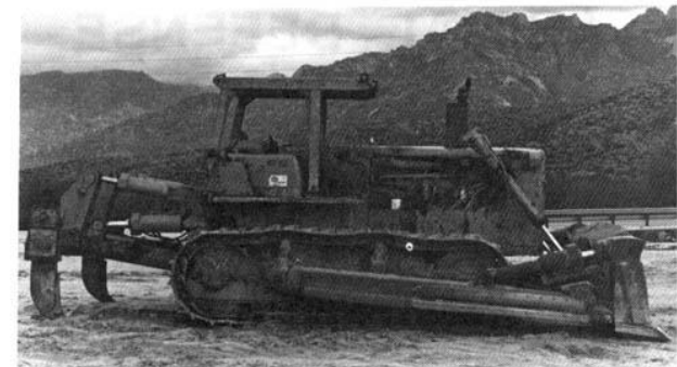
Bulldozer. Note the smoke stack (exhaust pipe).
